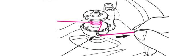
**5** Put the thread end into the guide at the bobbin winding shaft and pull it to the right side to cut it.
