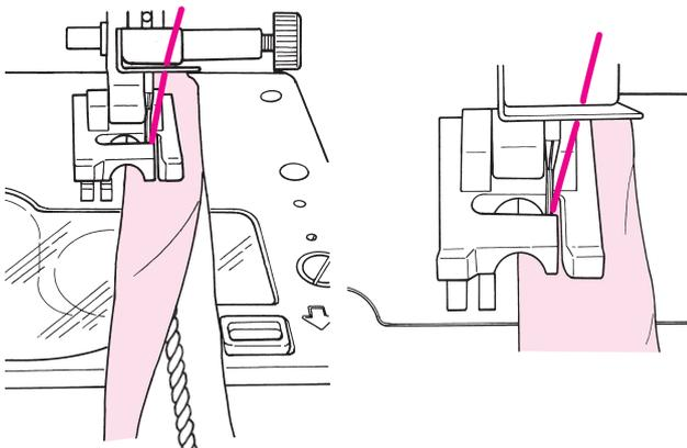
**2** Fold the cut fabric in half and wrap the cord. Sew the edge of the cord. Change the needle position to [7.0].
