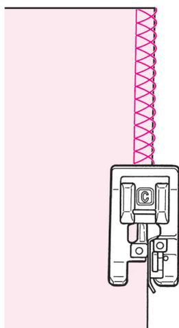
Push the fabric towards the guide and sew. If the fabric and guide are apart, it will not make a nice stitch formation. Make sure to guide the fabric along the guide and sew slowly.
