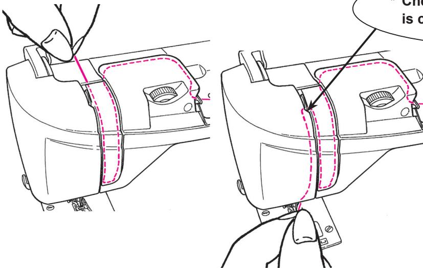
\* Check that the thread take-up is correctly threaded.
