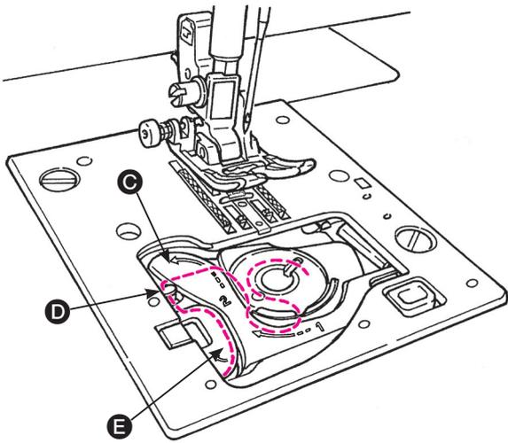
**4** Thread to guide **D** and **E** leave the thread underneath. (Thread guide **E** first and it will thread to guide **D** as well.)
