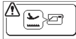
This means presser foot is up. Lower the presser foot to start sewing.
