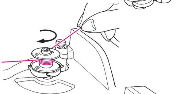
**4** Wind the thread to the bobbin 4-5 times in clockwise direction.
