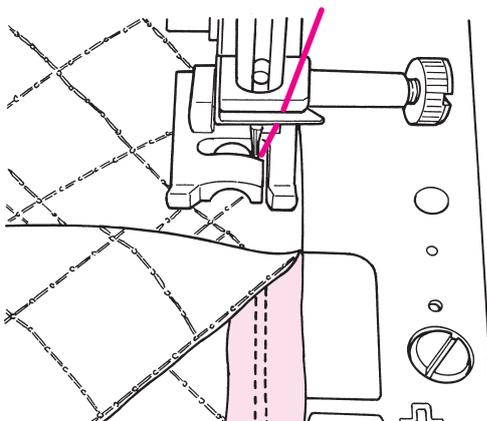
**3** Attach the piping core to a project. At this time, change needle position to [6.6] and sew as per 2 above, then stitches will not be on the right side of the fabric.
