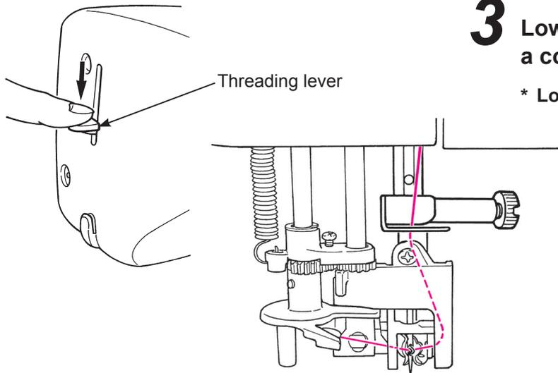
**3** Lower the threading lever until it comes to a complete stop.
