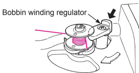
**7** When winding is finished, the shaft stops automatically, the bobbin winding regulator moves to right and return to the original position.
