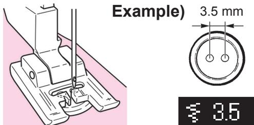
**2** Place a button under the presser foot and adjust the zigzag width according to the distance between holes in button.
