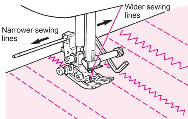
**2** Sew while tracing the stitches with the tip of the quilt guide.
