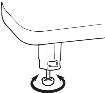
**4** Adjust the height of legs so that the top surface of Wide Table is the same height of sewing machine body.
