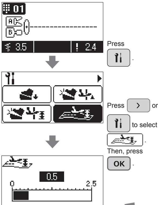
Press to adjust the presser foot to such a height that it holds the fabric appropriately.
