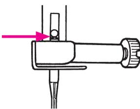
It is impossible to perform stitching if the needle is not correctly installed or a bent needle is used. Pay close attention as this will cause machine malfunction.
