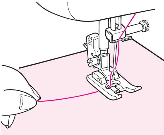
Pass down the needle thread through the presser foot hole and draw it sideways. Place the fabric underneath the presser foot and start.
