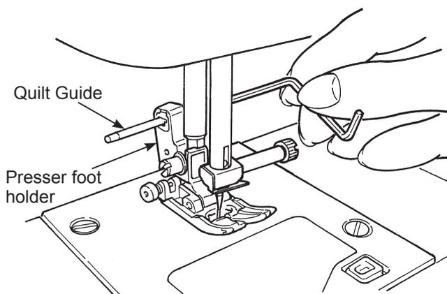
**1** Insert the quilt guide into the groove of the presser foot holder.
