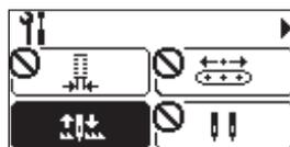
The twin needle setting can only be carried out when suitable pattern is selected and center needle position is selected at the same time.
