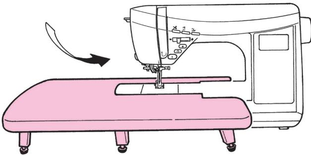
**3** Assemble Wide Table to sewing machine body.
