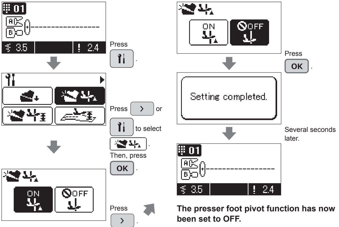
\* The setting is memorized even when the machine is turned off and on.
