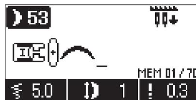
**Symbol of twin needle sewing will be shown on the display.**
