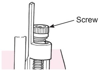
**4** Turn off the machine and adjust the height of the presser foot with adjusting screw.
