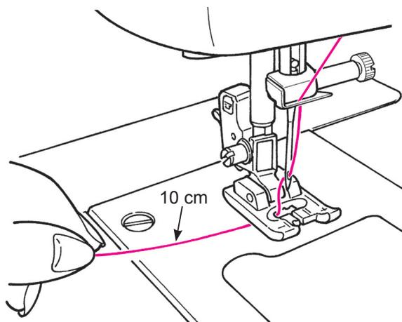
**1** Pass the needle thread through the presser foot.
