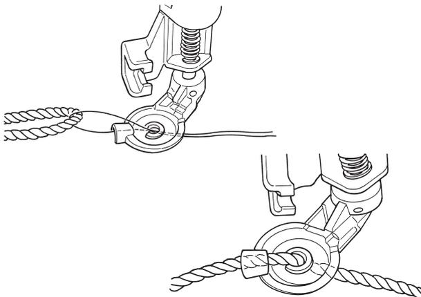
**2** Using wire, pass the cord through the hole of the presser foot.
