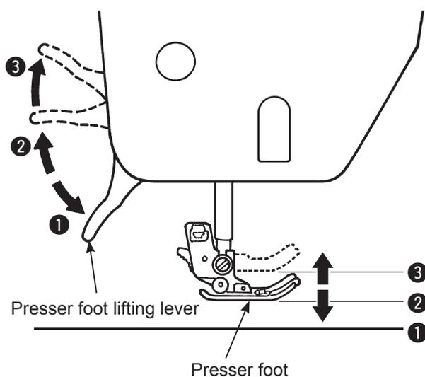
The presser foot is lifted/lowered with the presser foot lifting lever.
