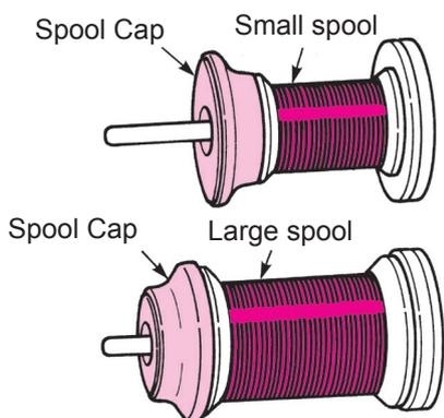
**1** Place a thread spool to spool pin and a spool cap onto the spool pin.
