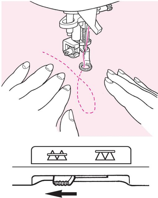
**4** Place the fabric underneath the presser foot and lower the presser foot.
