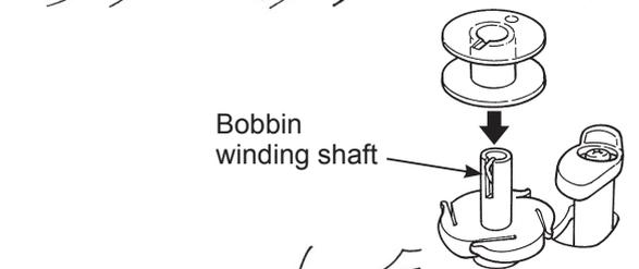
**3** Set the bobbin on the bobbin winding shaft.
