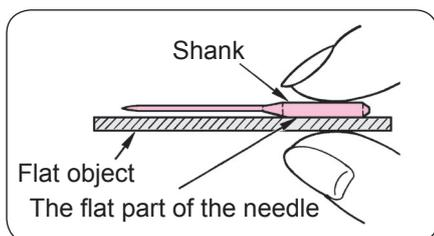
Check the needle for its straightness occasionally. Any bent needle would cause skipped stitches, thread breakage or damage to materials.
