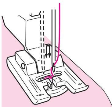
**4** Carry out sewing while turning the handwheel by hand.
