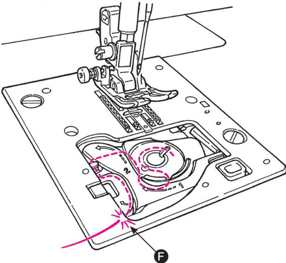
**5** Cut the thread with the built-in cutter **F**.
