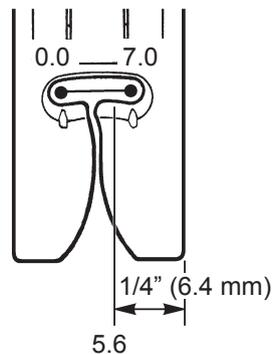
The needle position can be adjusted between 0.0~7.0.
