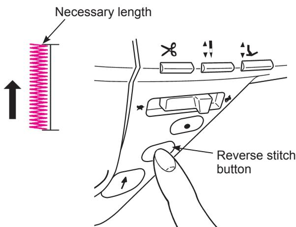
Push the reverse stitch button when it reaches the necessary length of the left side of the buttonhole.
