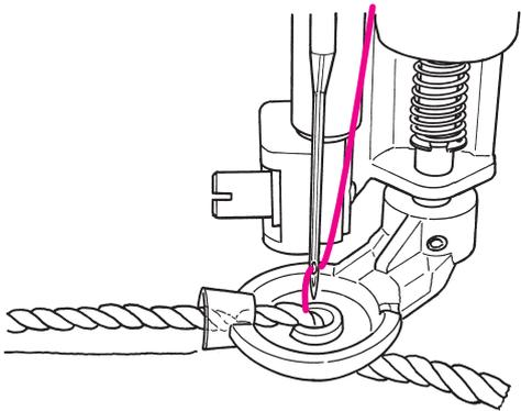
**5** Sew 2 - 3 stay stitches to fix the cord to the fabric. Adjust the needle position if necessary. (Make sure to check that the needle will not hit the foot.)
