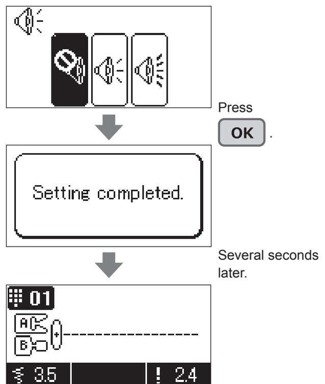
**Now the volume setting is changed and it will not produce a sound even when a button is pressed.**
