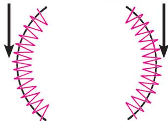
Keep the needle inside the fabric at the point of arrow and raise the presser foot.
