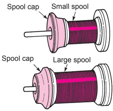
There are three types of the spool caps, large, medium and small. Choose the size of spool cap according to thread spool to be used.
