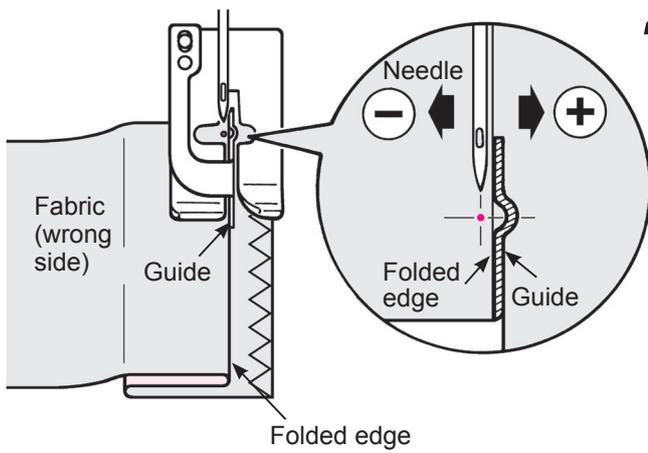
**4** Align the guide of the presser foot with the folded edge.
