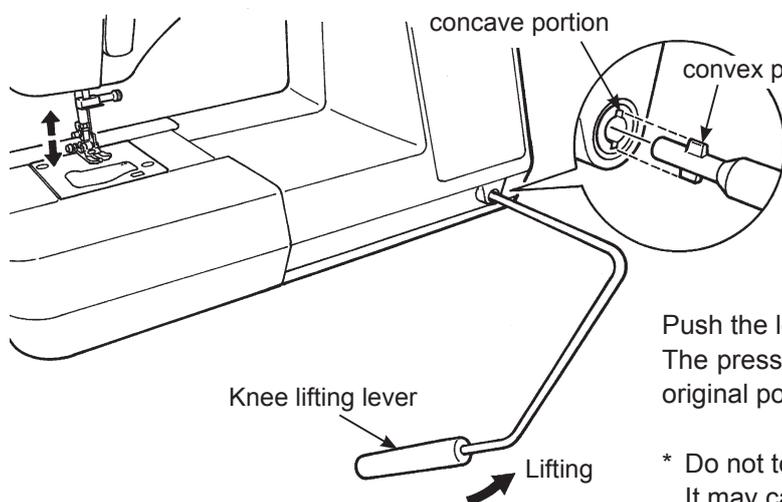
Insert the knee lifting lever so that concave and convex meet.
