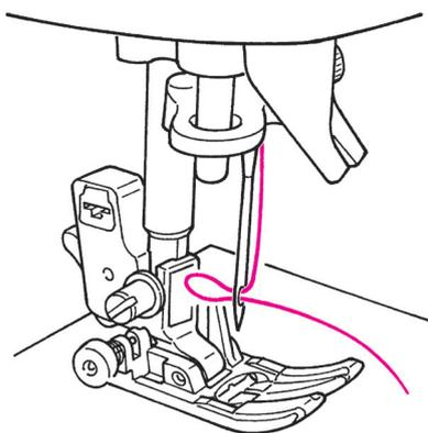
**4** Release the threading lever and the needle thread is threaded to the needle eye.
