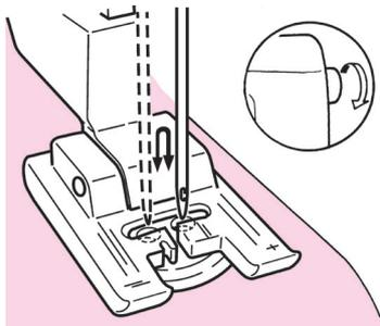
**3** Make sure that needle enters holes in button, by turning hand wheel manually.
