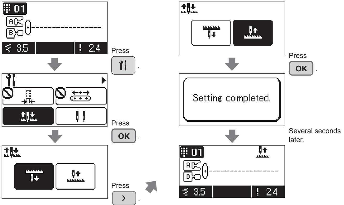
**The needle stop position is set to the needle-up stop.**
