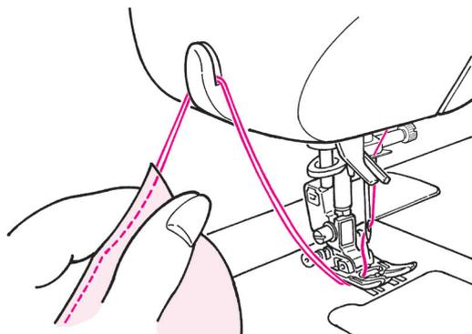
\* You can also cut the threads by the thread cutter at the face plate cover.
