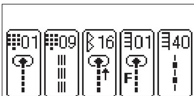
After you have changed the needle hole to the needle hole for straight stitches, press
