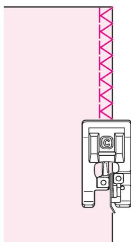
This stitch is used for overcasting medium- to heavy-weight materials. Guide the fabric along the guide and sew.
