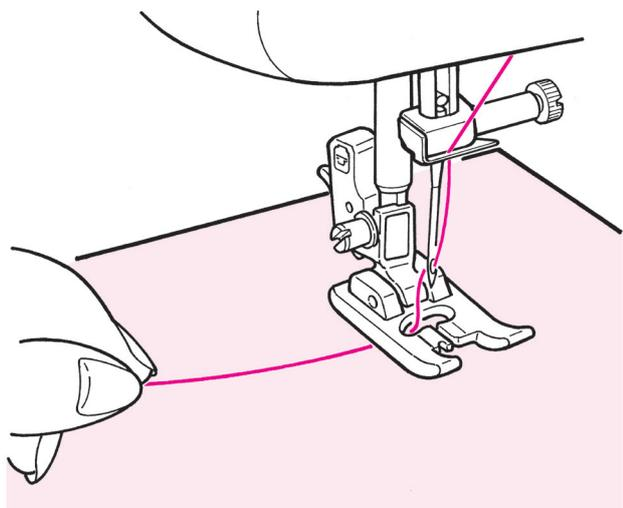
Pass down the needle thread through the presser foot hole and draw it sideways. Place the fabric under the presser foot and start.
